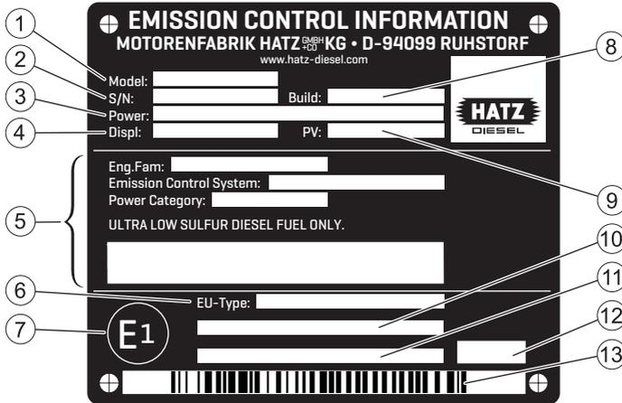
The engine type plate is affixed to the crankcase and includes the following engine information:
