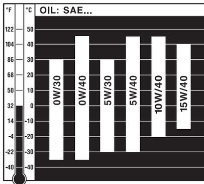
Select the recommended viscosity depending on the ambient temperature at which the engine will be operated.
